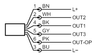
OUT1: IO-Link / switching output
